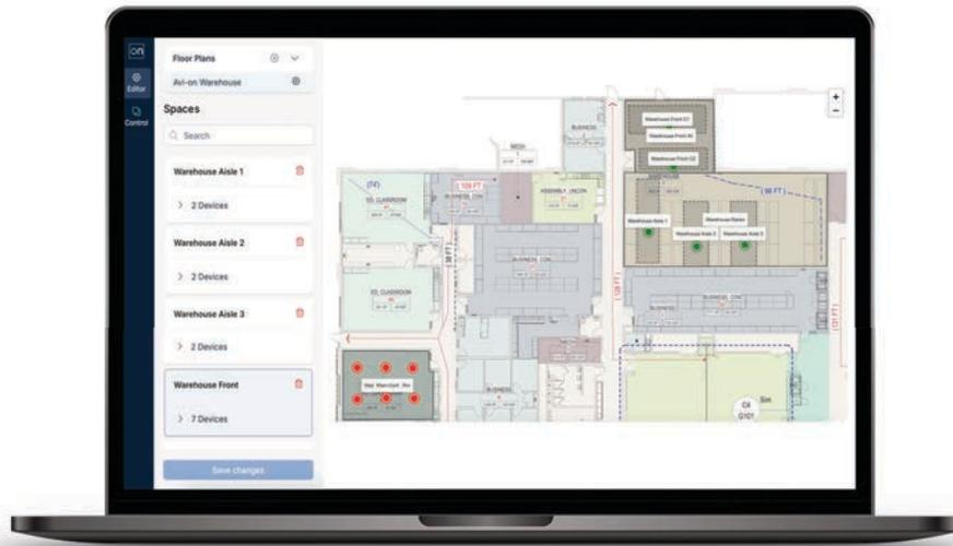
Avi-on has released a web based control capability to turn devices and rooms on and off from a floorplan based web browser interface. To control an area, the user uses the web browser interface to navigate to the area they want to control. The browser is managed by the Avi-on cloud to allow control from any location. An Avi-on RAB LTE is required to connect the local Avi-on BLE network to the Avi-on cloud. Both LTE and Ethernet connectivity are supported.
